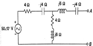
Q.4 a) Find v, dv/ dt &  $d^2v/dt^2$  for following circuit.
